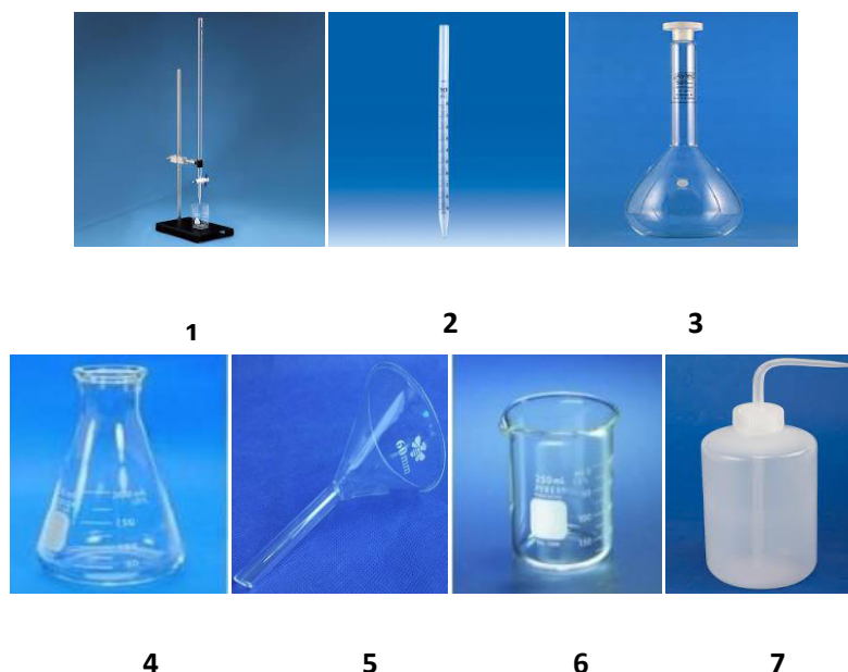
Fig.34. Components of a Titration Assembly
