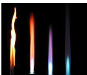
Fig.16.3. Bunsen burner flames depend on air flow in the throat holes
